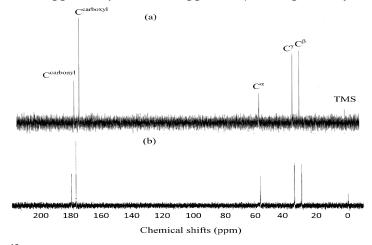
**Figure 3:** <sup>13</sup>C NMR spectra of  $\gamma$ -pga (a) and [Zn( $\gamma$ -pga)] complex (b) in D<sub>2</sub>O. The <sup>13</sup>C spectra were recorded downfield from 0.00 ppm using tetramethylsilane (TMS) as an internal reference.
