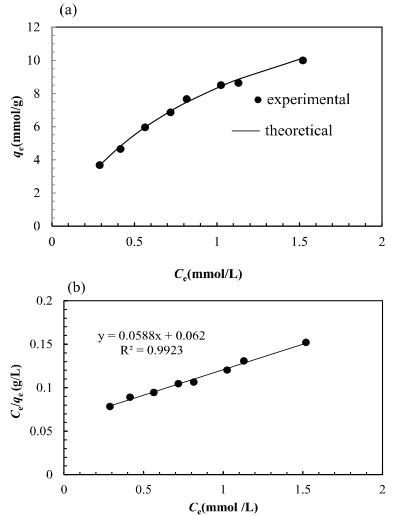
**Figure 4:** Binding isotherm (a) and the corresponding linearized plot (b) for the chelation between Zn(II) ions and  $\gamma$ -pga at pH 5 and temperature 30 °C. The theoretical solid line in Figure 4(a) was generated by using the Langmuir model equation (2) and the values of  $a_L$  (0.94 L/mmol) and  $K_L$  (16.13 L/g) obtained from Figure 4(b).
